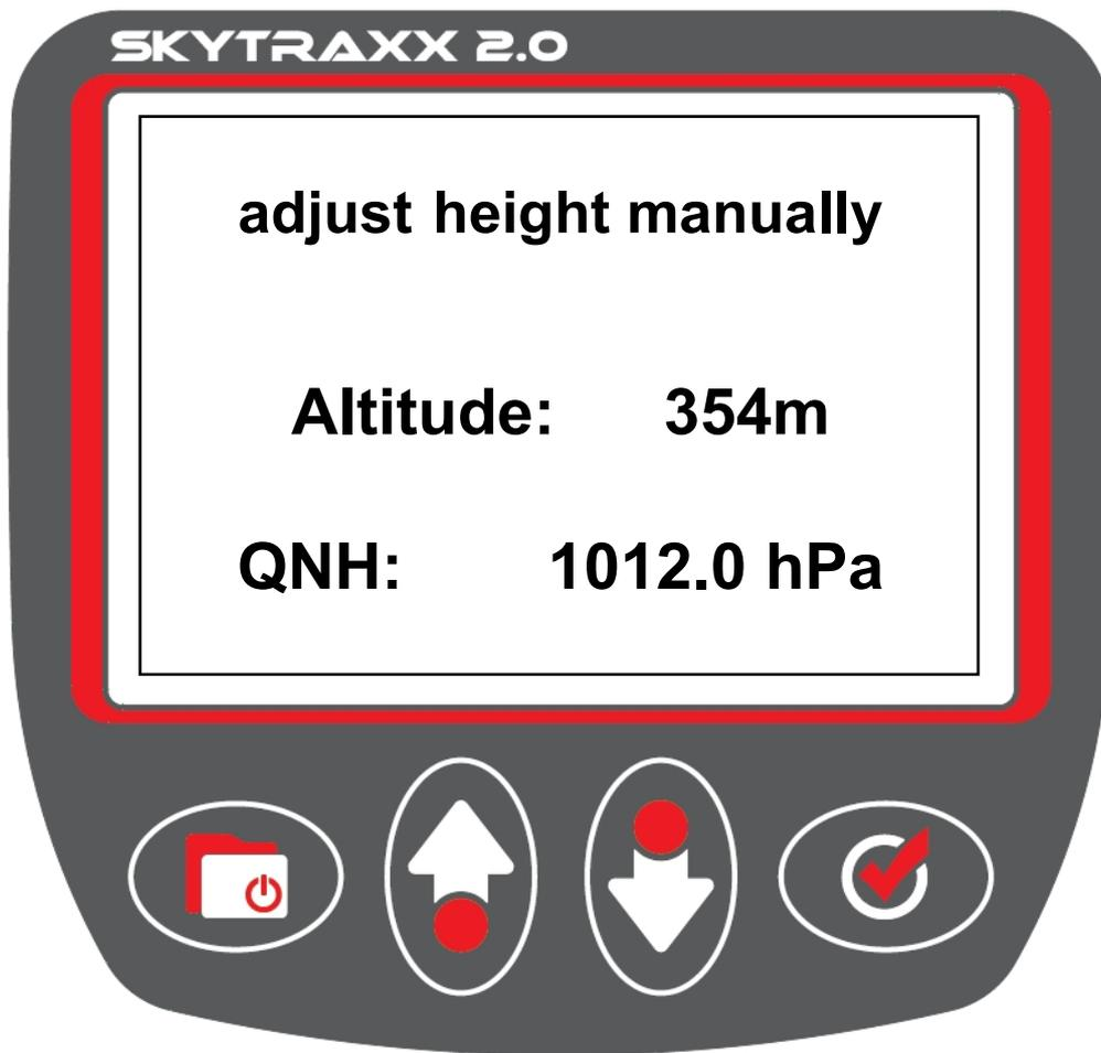
To manually set the altitude, press one of the middle keys whilst viewing the **Main Screen**. Adjust the values using the middle keys. Confirm by pressing **OK**.
