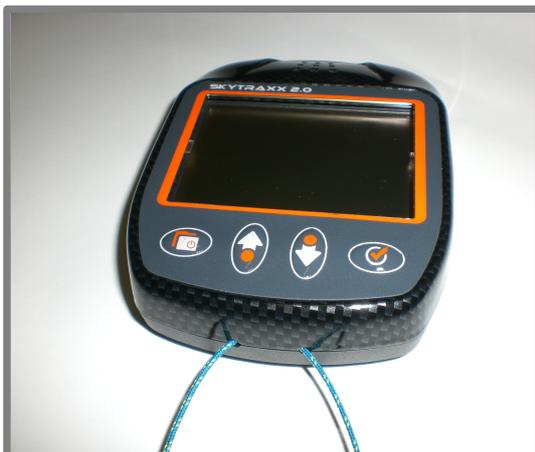
For in-flight security, a safety line can be attached using the two holes at the base of the unit.
