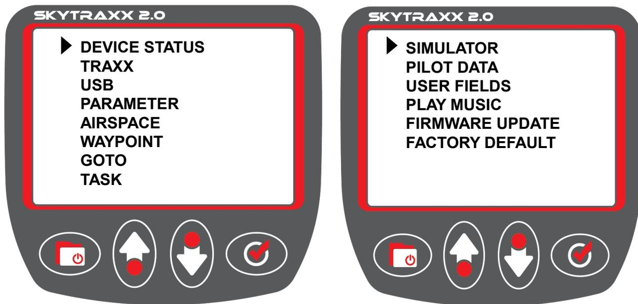
Use the **Minus/Plus** keys to move the indicator up and down the list (2 pages). Press the **Menu** key anytime to return to the main screen. Press **OK** to open an indicated screen.
